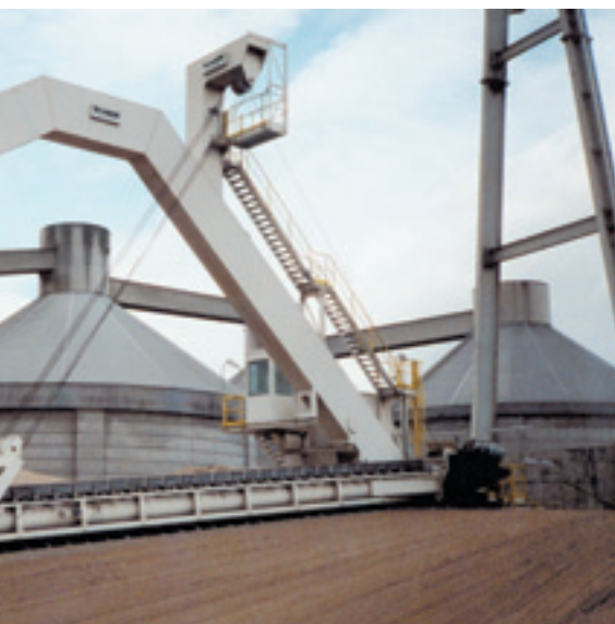
Type Reclaimer in outdoor stockyard
