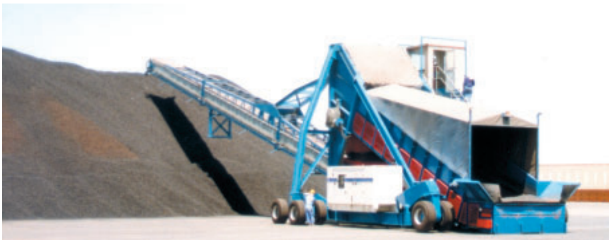
Stormajor stockpiling various materials from wood chip to iron ore for a Middle East steel works stockyard
