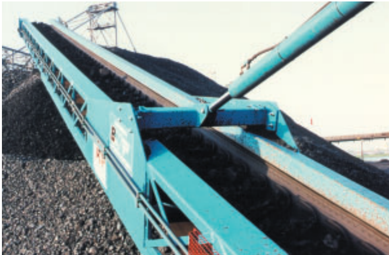
Cantilevered Outloading Boom with Slew Ring Mount and Hydraulic Actuator
