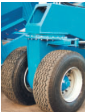
Twin Axle Steering Bogie with potentiometer alignment system to achieve Ackerman steering without a mechanical linkage.
