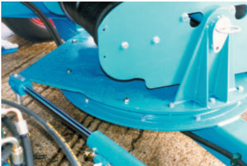
Cantilevered Outloading Boom with Slew Ring Mount and Hydraulic Actuator
