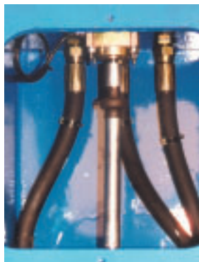
Rotary Potentiometer linked to the slew ring determines the wheel orientation and maintains both steering wheels in correct alignment using an electronic comparator system.
