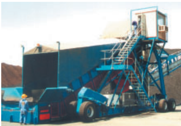
Control cabins may be mounted at high level as shown above or at low level on the main chassis - see page 20
