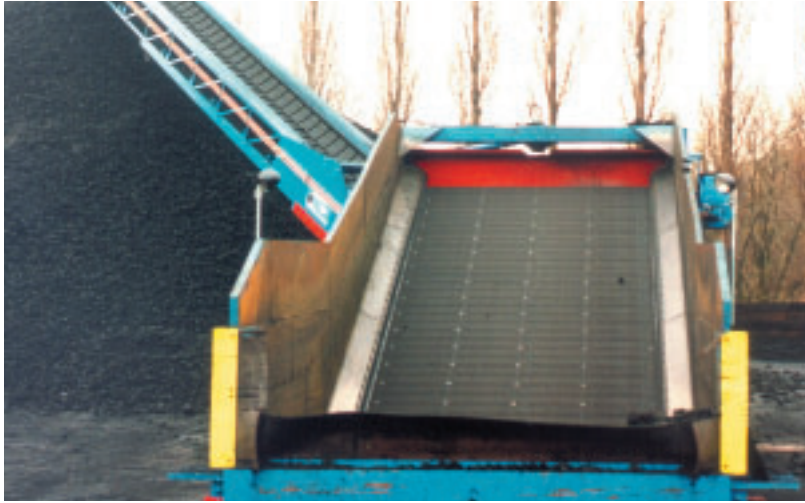
Stormajor handling smokeless fuel briquettes direct from tipping trucks
