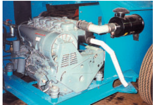
Deutz Diesel Motor with direct coupled hydraulic drive mounted beneath the Samson® inclined section
