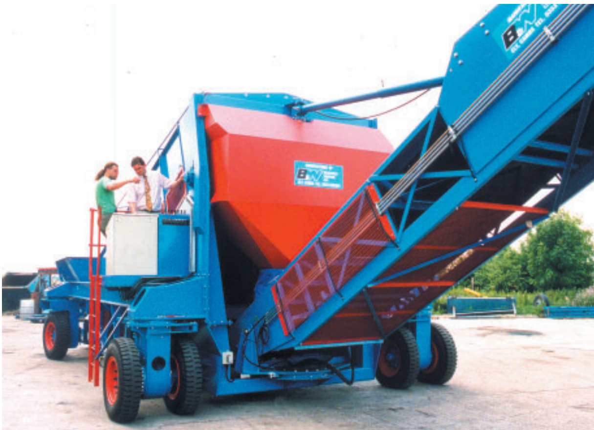
Wheel units are mounted to a slew ring with hydraulic actuators to control the wheel alignment from the drivers control position using a Joy-Stick controller linked to variable proportional hydraulic valves allowing variable travel speed
