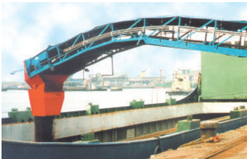
Extended Trimming chute showing also the full boom enclosure using flexible PVC covers
