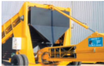
Stormajor handling smokeless fuel briquettes direct from tipping trucks
