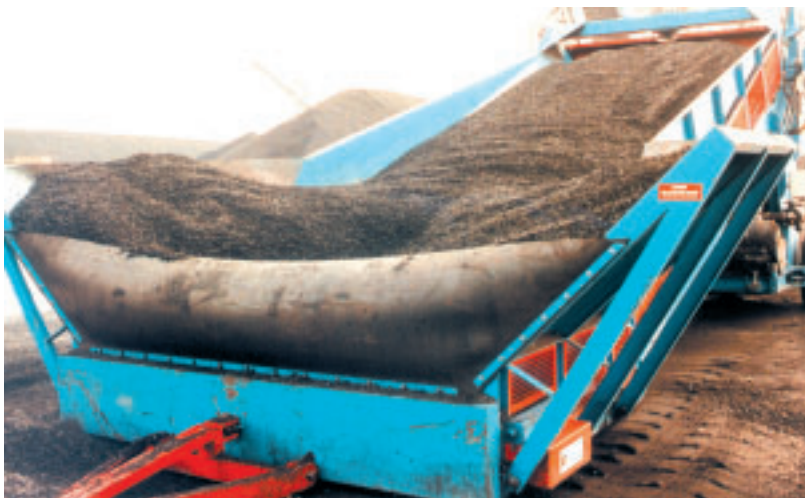
Stormajor receives coal from Loading Shovel for stockpiling and barge loading
