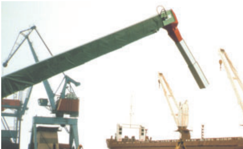
Extended Trimming chute showing also the full boom enclosure using flexible PVC covers
