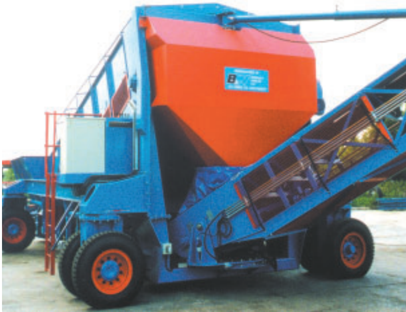
Wheel units are mounted to a slew ring with hydraulic actuators to control the wheel alignment from the drivers control position using a Joy-Stick controller linked to variable proportional hydraulic valves allowing variable travel speed
