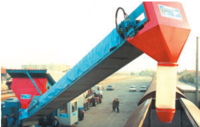
Outloading Boom with hydraulic head shaft drive shown here with full enclosure system - loading sand to rail wagons
