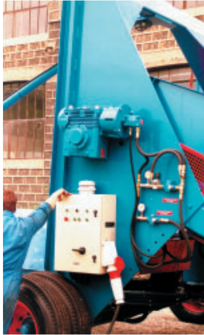
External control panel for electric motor drive with detachable cable
