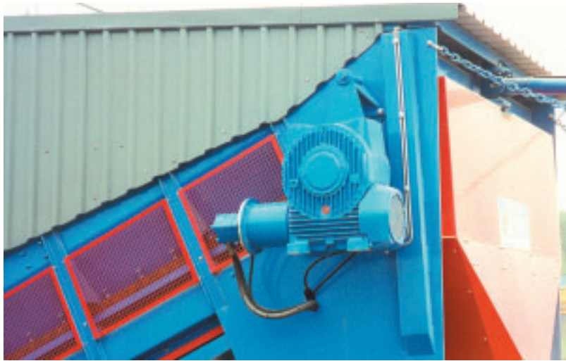
Drive to the Samson® receiving section by direct coupled hydraulic motor with a shaft mounted worm reduction gear
