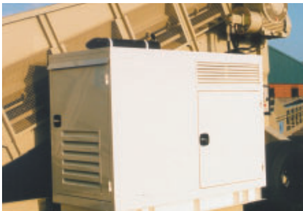
Diesel motor drive with triple section hydraulic pump system fitted to the side of the main chassis within a sound attenuated enclosure
