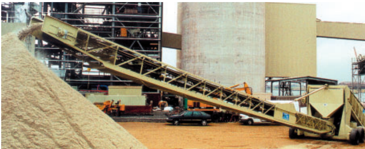
Stormajor Stockpiling Granulated Steel Slag direct from tipping trucks
