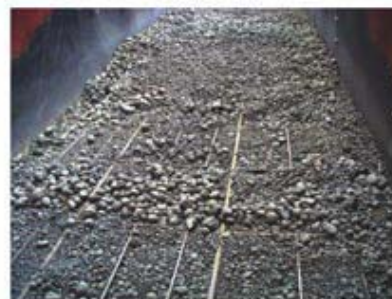
Cold clinker protects against hot material
