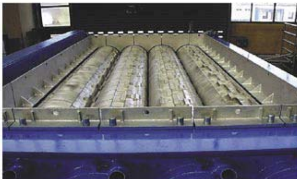
A roller crusher for a 4,200-t/d operation
