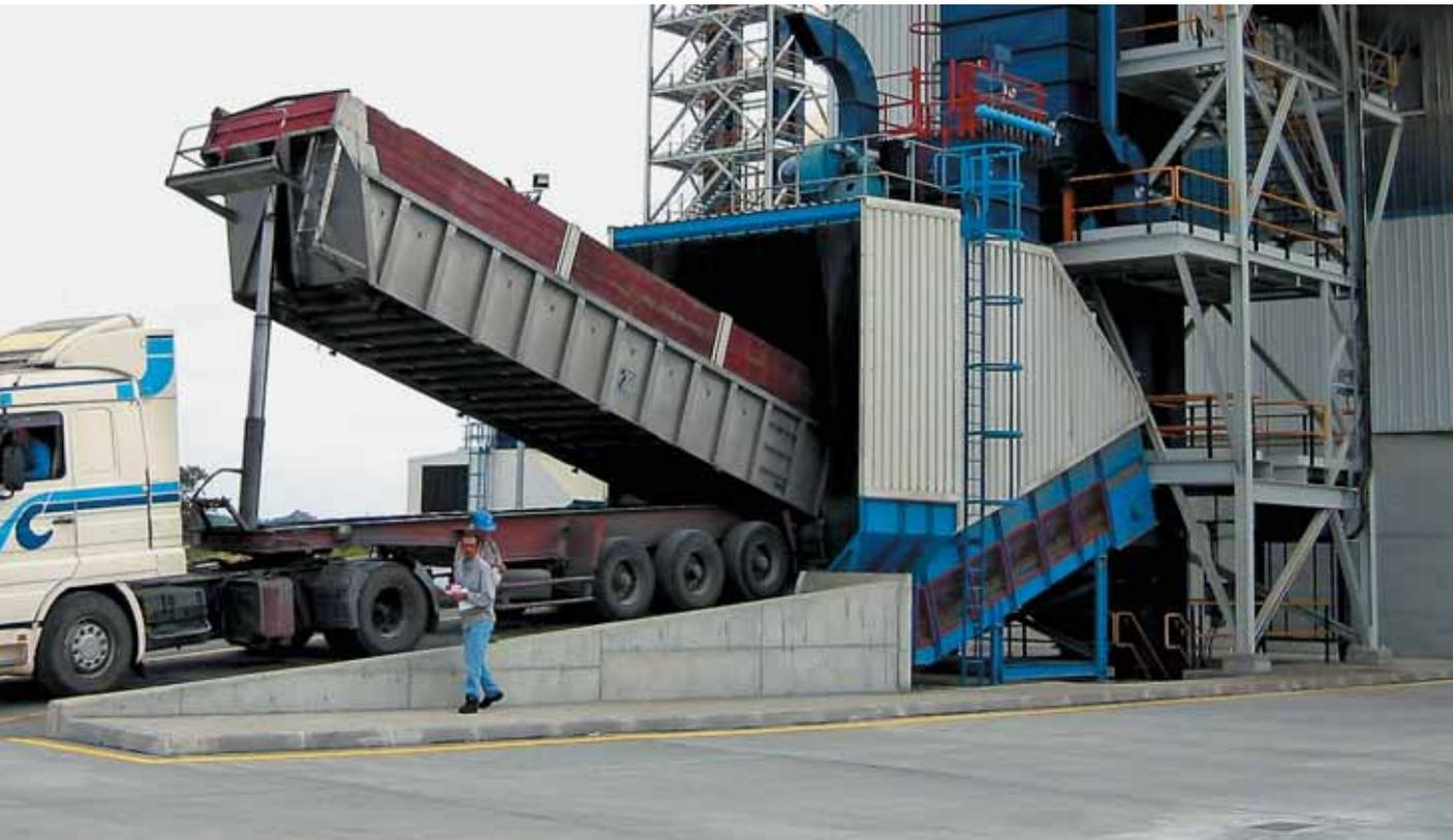
Samson® Surface Feeder – Coal and Petcoke Intake
