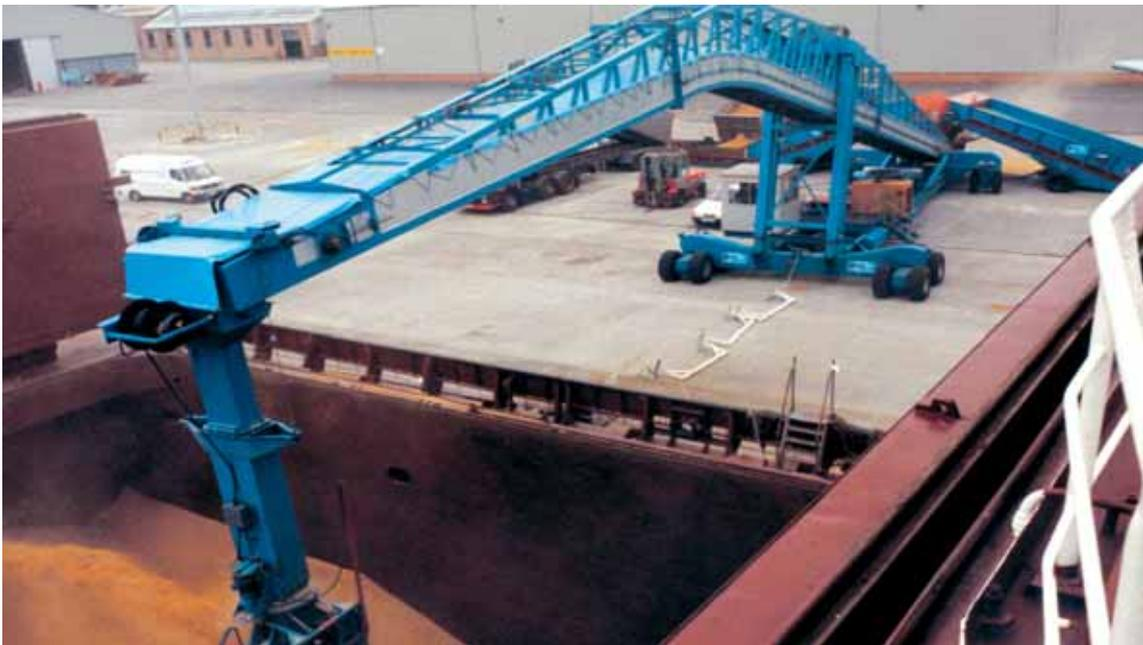
Mobile Shiploader with Samson® Surface Feeders - Direct Transfer from Truck to Ship
