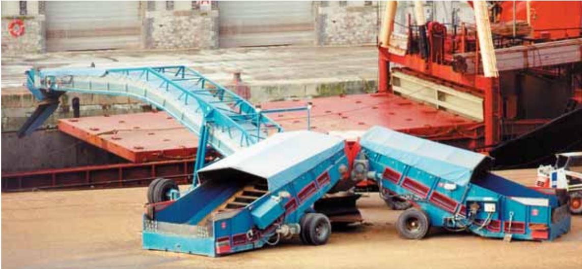
Twin Independent Samson® Feeders Discharge to a Single Shiploader
