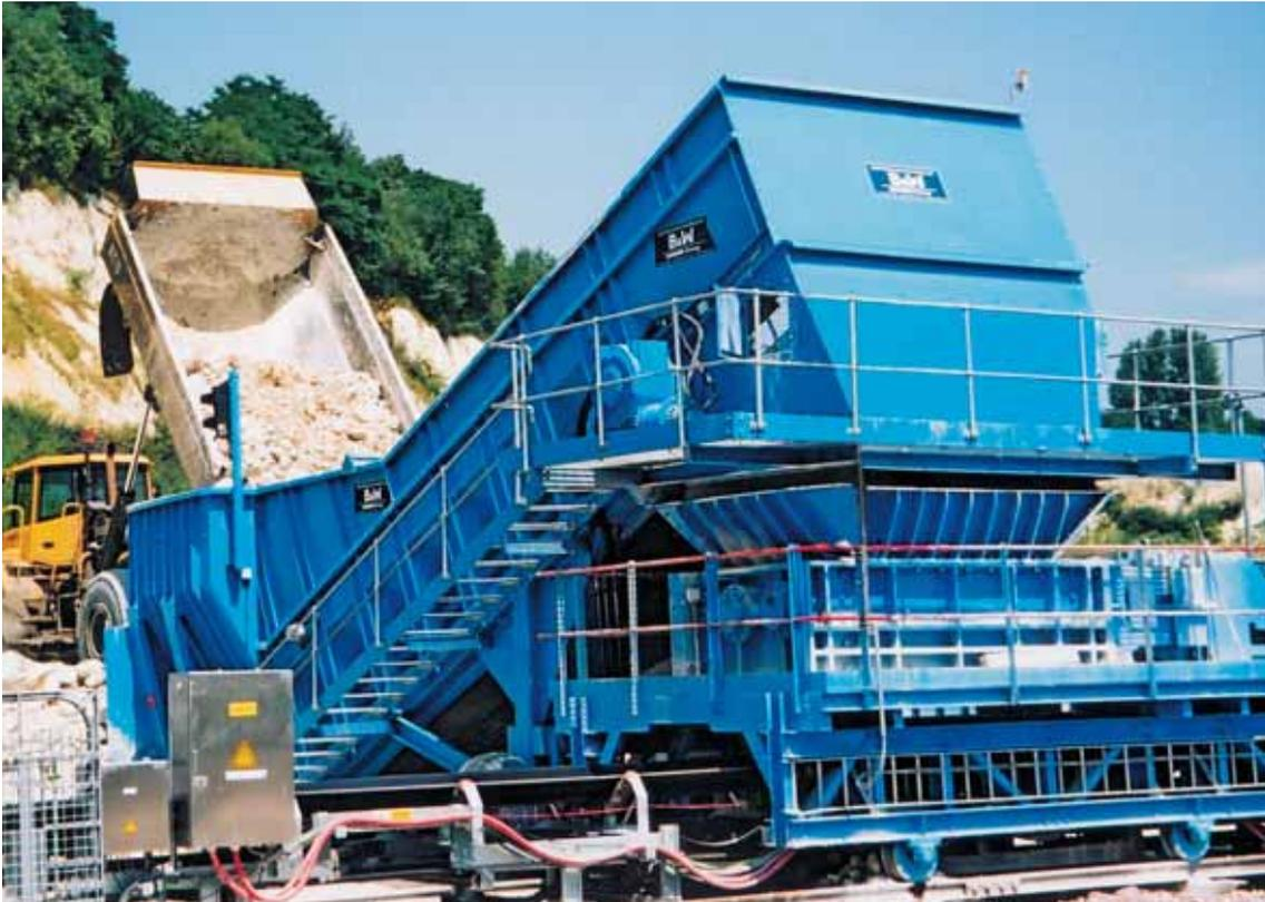
Samson® Surface Feeder with Integrated Crusher
