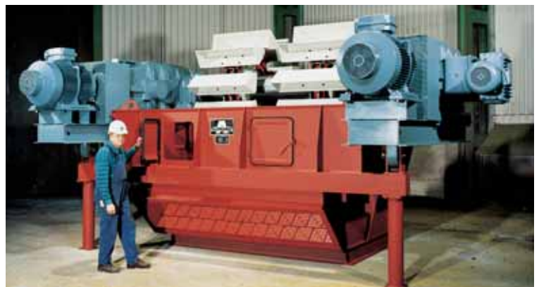
Double Bucket Elevator for a conveying capacity of 1,300 t/h
