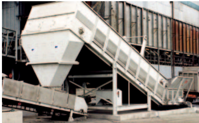
The Samson™ with a Centralising Head Chute discharges to a conveyor positioned In-Line
