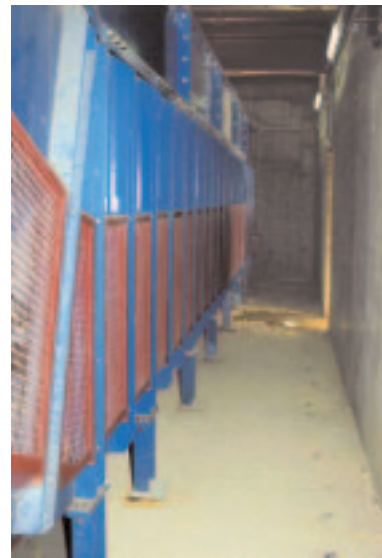
Discharge facility for Hopper Bottom Railcars receives coal for a Cement Plant including a Samson™ feeder with 80 tons holding capacity
