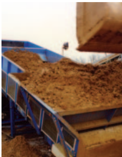
The Samson™ with Straight Chassis and Flared Entry (width 4.5 m) receives Sandy Clay from Shovels
