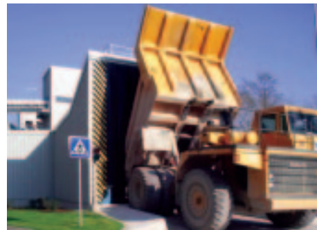
Twin Rotor Sizer supplied with the Samson™ 1600 Series feeder receives ROM Limestone for crushing down for onward conveying
