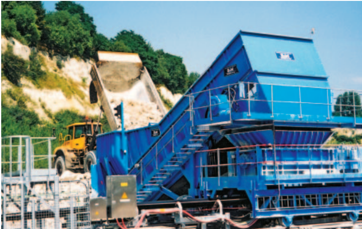
Twin Rotor Sizer supplied with the Samson™ 1600 Series feeder receives ROM Limestone for crushing down for onward conveying
