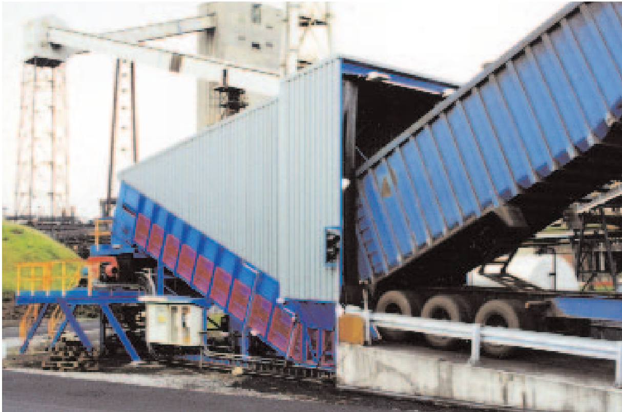
The Samson™ Receives Coal for the Coking Plant at a major UK steel works operating continuously 24/7
