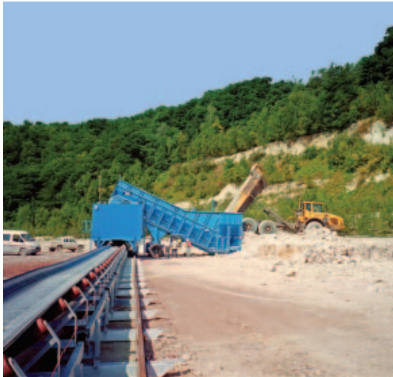
Mobile Samson™ in Quarry with Integral Sizer receives from Dump Trucks
