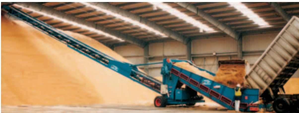
The B&W Stormajor™ combines the benefits of a Samson™ Surface Feeder with a Radial Stacking Boom mounted to a common mobile chassis.
