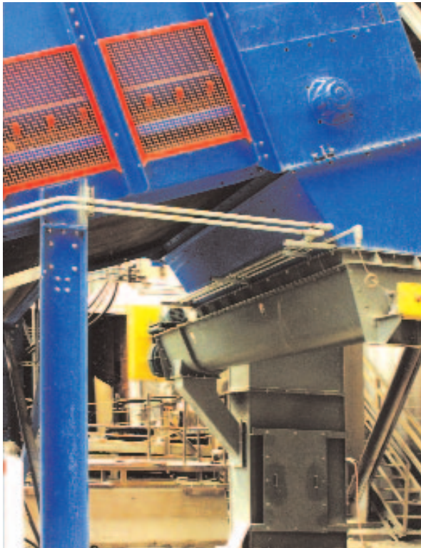
Single Screw Feeder provides metered output to a Bucket Elevator
