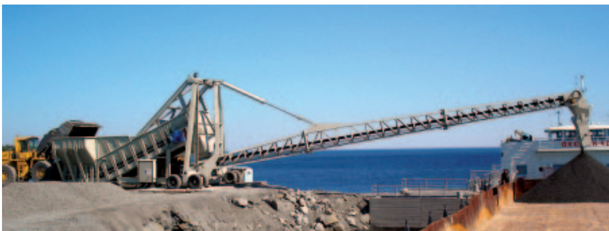
The B&W Stormajor™ with integrated Samson™ 1600 Series Feeder and Radial Stacking Boom for Barge Loading
