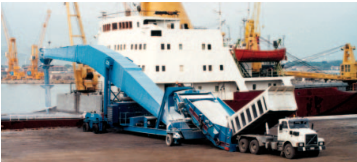
The Samson™ Feeder integrated to this Mobile Shiploader permits direct bulk export from Truck to Ship
