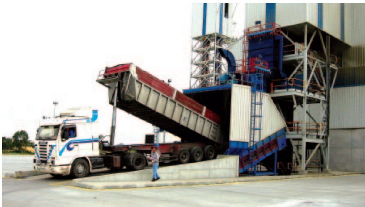
In this Cement Grinding Plant three Samson™ Bulk Material Receiving Units intake Cement Clinker plus other additives for the whole plant
