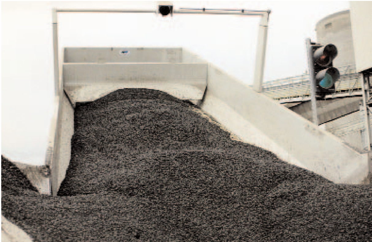
Material Stored within the Samson™ body may be at various Load Levels along the length of the Samson™
