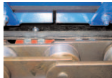
Load Carried on the Chain Rollers
