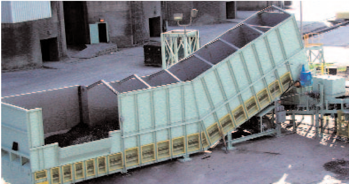
The Samson™ 800 Series provides 100 cubic metres of live storage for Alternative Fuels in a Cement Plant.
