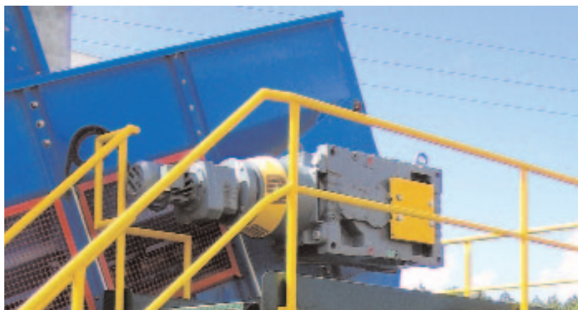
High efficiency Helical/Bevel main reduction gear with helical primary
