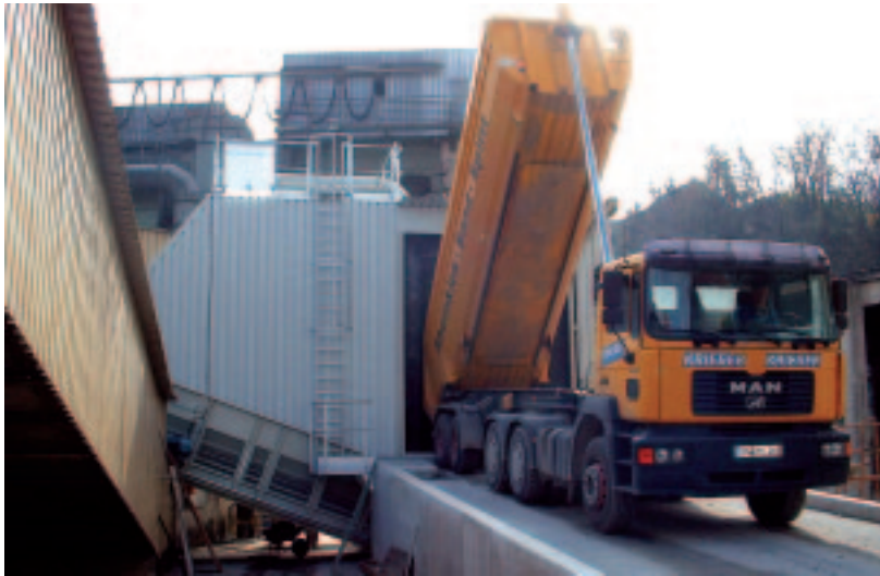
The Side Loading Samson™ receives Cement Clinker for import directly to an existing conveyor installation
