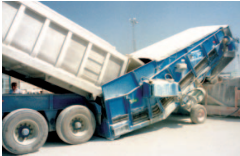
Mobile Samson™ Feeder receives Kaolin for Ship Loading (Truck to Ship Concept)
