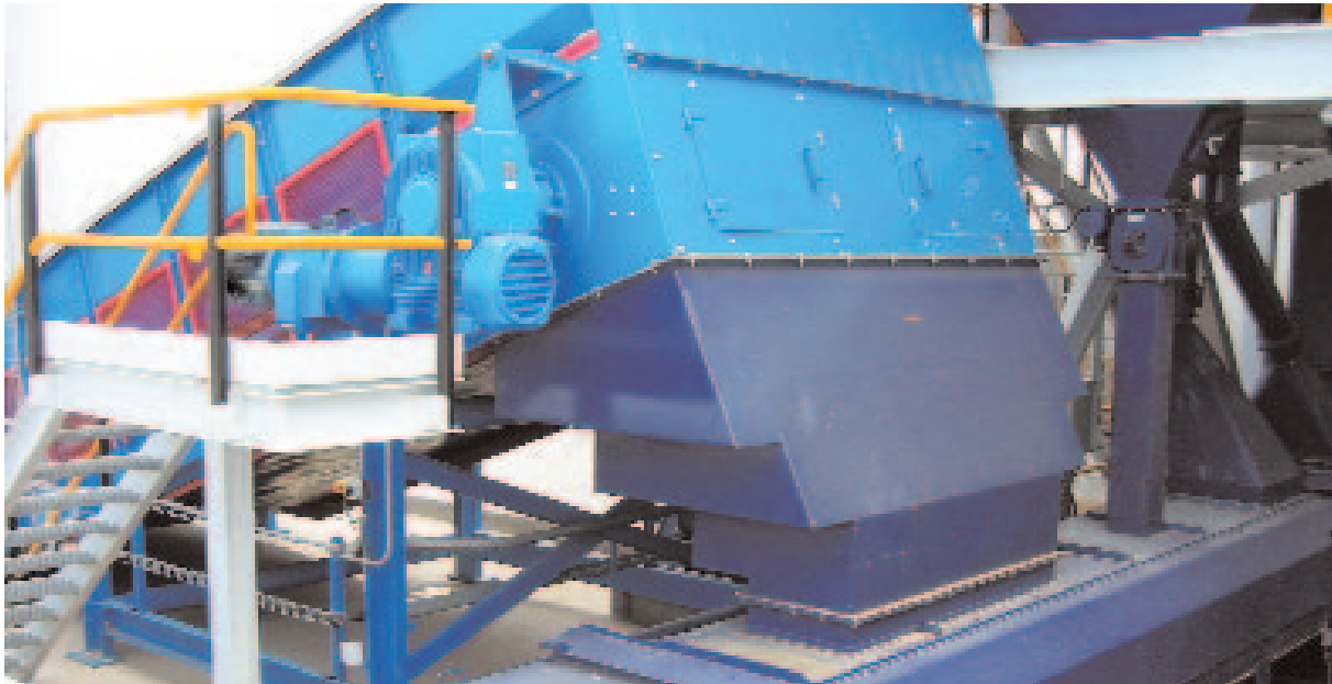
All Samson™ Feeders are supplied as standard with a shaft mounted reduction gear
