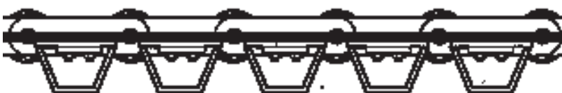
Conveyor Belt Aligned with the Chain Pin Centre and Rivetted to the Steel Apron Bars
