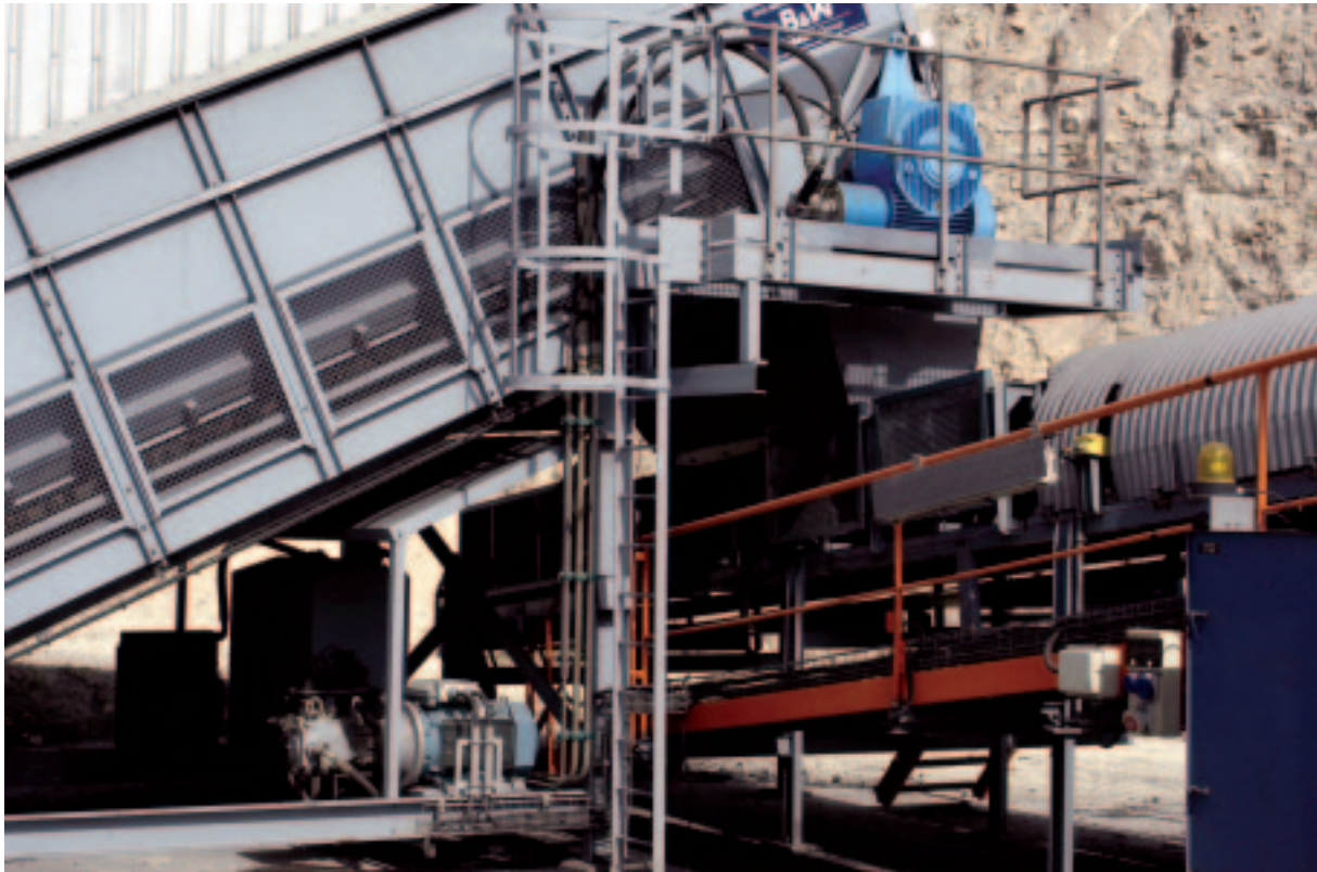
Hydraulic Drive comprising Variable Displacement Hydraulic Pump providing local or remote belt speed control
