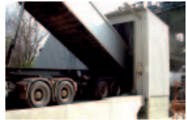
The Side Loading Samson™ receives Cement Clinker for import directly to an existing conveyor installation
