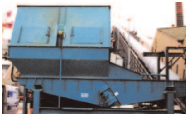
Vibratory Feeder provides regulated output to an inclined belt conveyor
