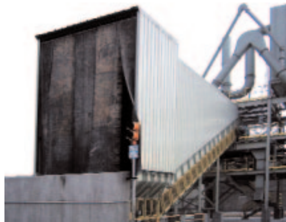
Extended Inclined Section for increased storage or discharge height
