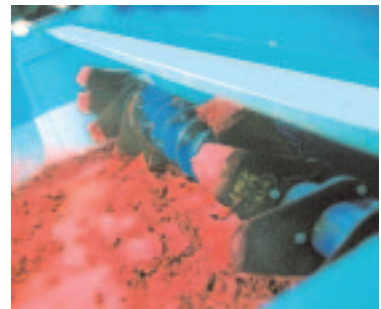
Levelling Blade controls the material bed depth at the Samson™ Discharge
