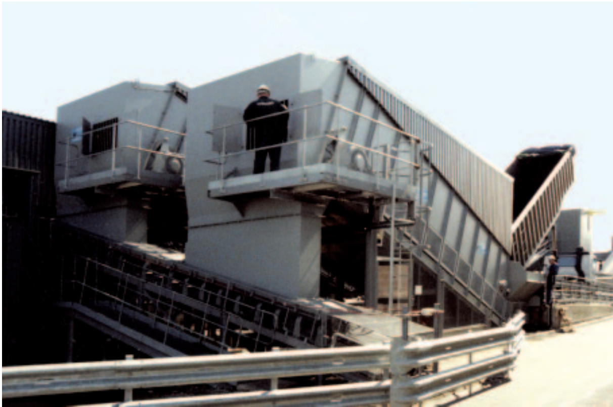
Twin Samson™ Surface Feeders discharge to a Common Belt Conveyor at 90 degrees with Parallel Chutes
