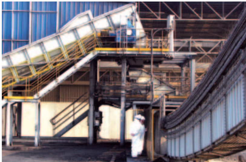
Samson™ supplied with Vibrating Screen to remove oversize material before onward conveying
