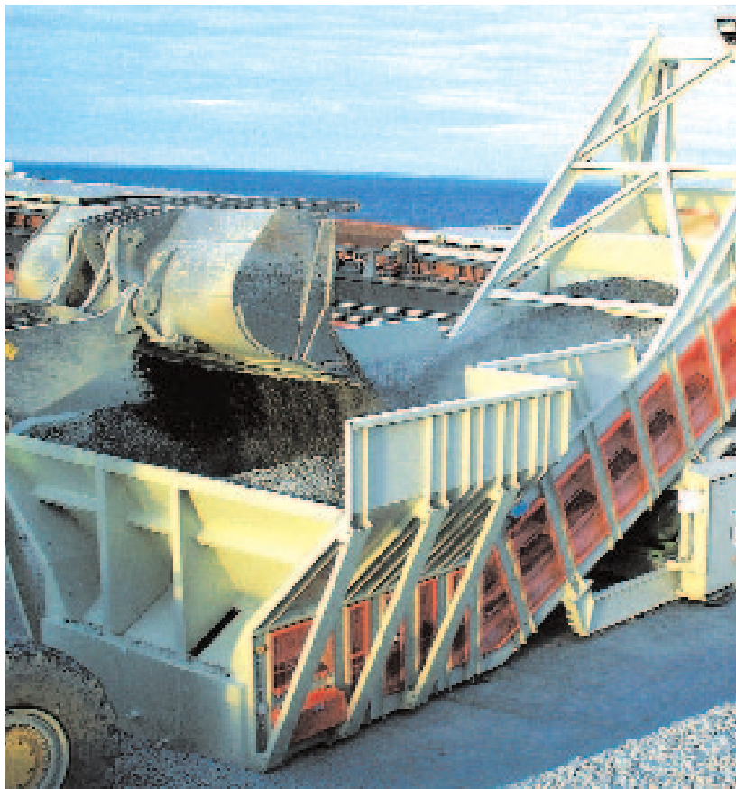
The Massive Samson™ 1600 receives Gabbros Rock from Shovels for Barge Loading at 1,000 t.p.h.
