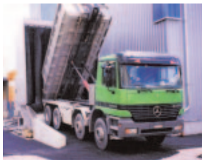
The Samson™ receives Sand for a Mortar Plant discharging to Belt Transfer Conveyor
