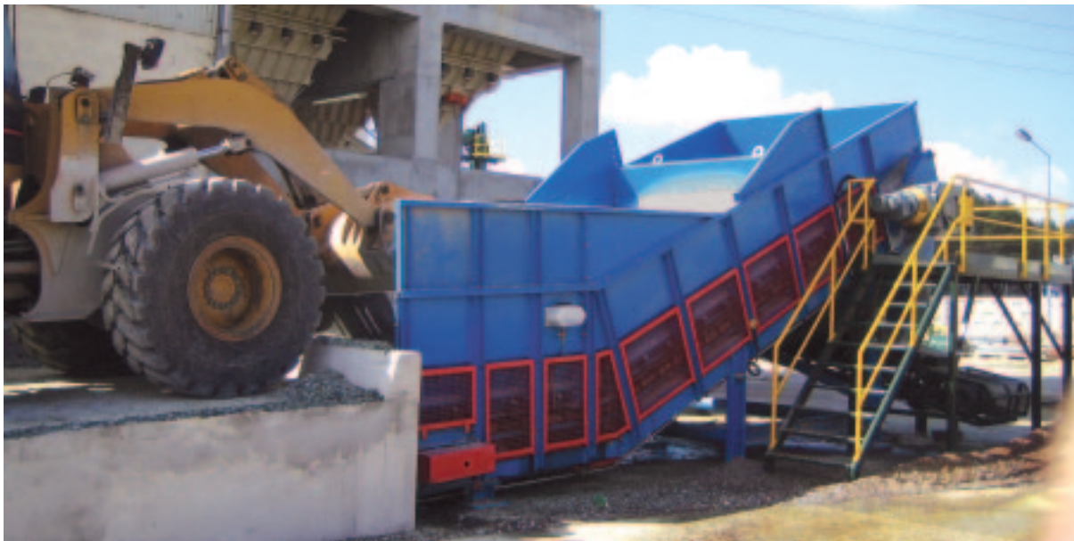
The Samson™ with Deflected Chassis and Parallel Entry (width 3.0 m) receives Broken Glass from both Tipping Trucks and Shovels
