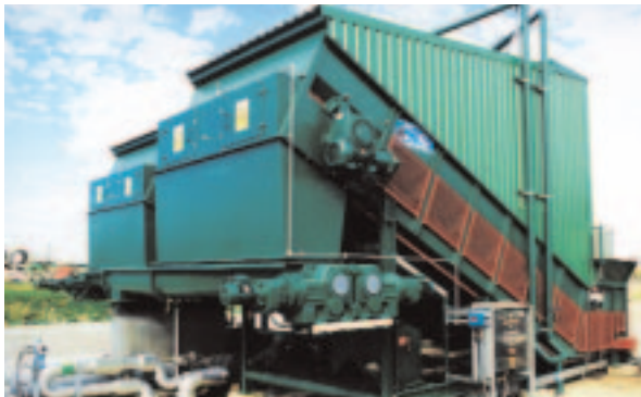
Twin Screws meter output to Progressive Cavity Pump
