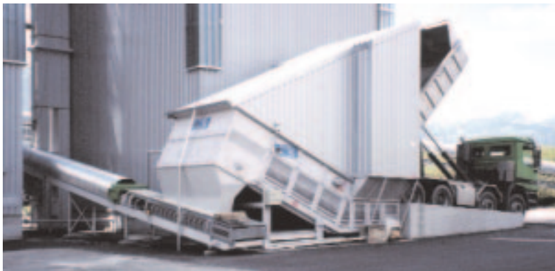
The Samson™ receives Sand for a Mortar Plant discharging to Belt Transfer Conveyor
