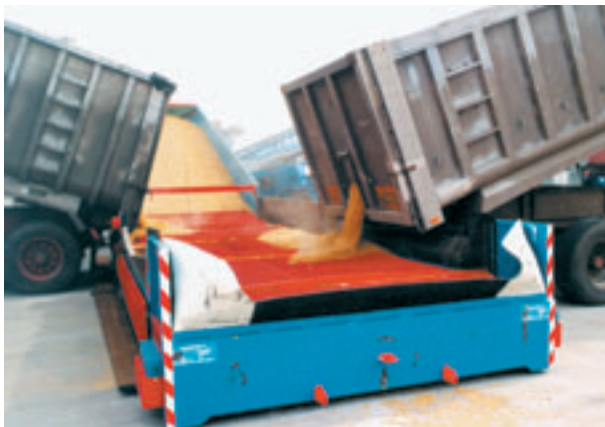
Up to four trucks discharge simultaneously per Samson® feeder
