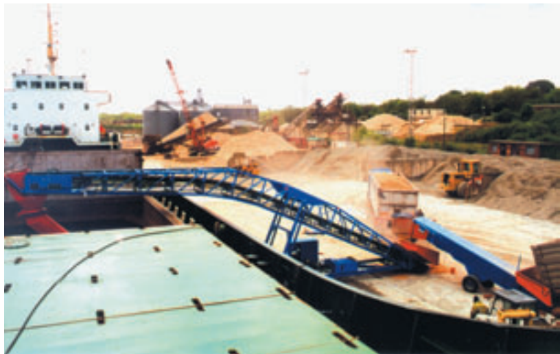
Feeder Conveyors discharge to the Shiploader
