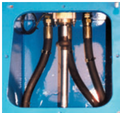
Rotary Potentiometer linked to the steering system provides automated wheel alignment in any travel mode
