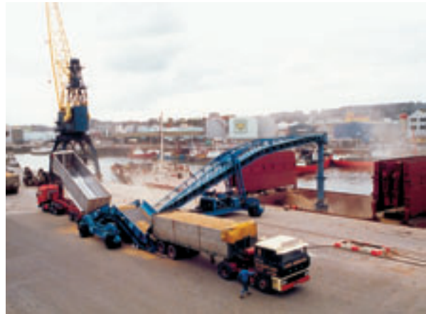
Twin integral Samson® feeders mounted to the Shiploader chassis
