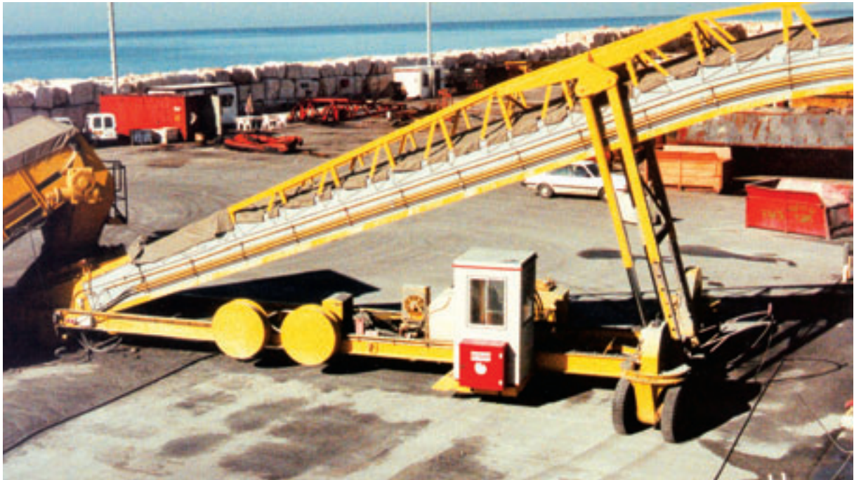
Powered Radial Operation with In-Line Tow Travel
