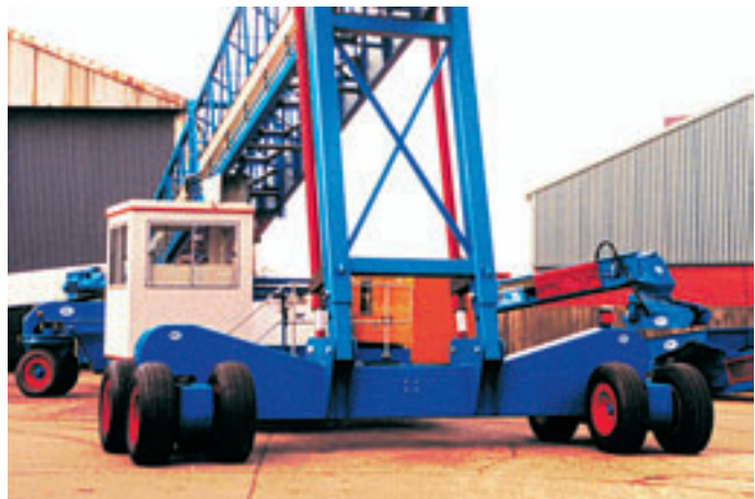
Forward Axle Beam with Telescopic Boom Supports
