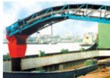
Variable Angle Trimming Chutes handle wet and sticky materials illustrated above loading FGD Gypsum and Peat.
