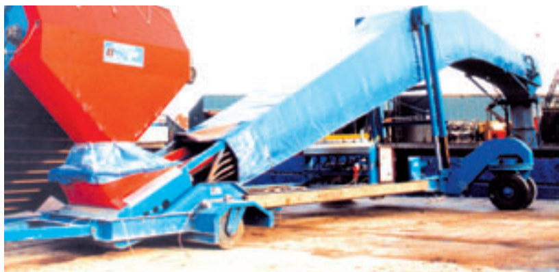
Tail end Castor-Wheel mounts with Parallel Push Travel
