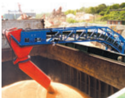
Rotating Variable Angle Chutes offer an economical solution with accurate trimming capability
