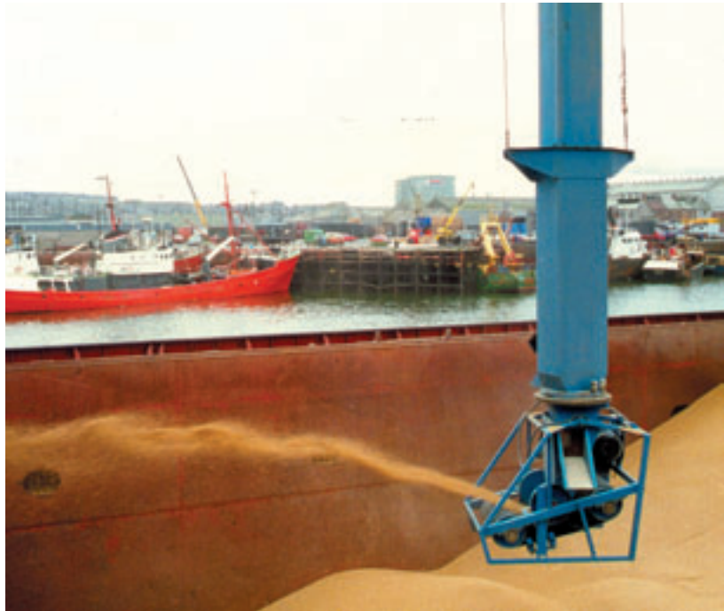
Radial Thrower provides effective trimming with minimum machine movements
