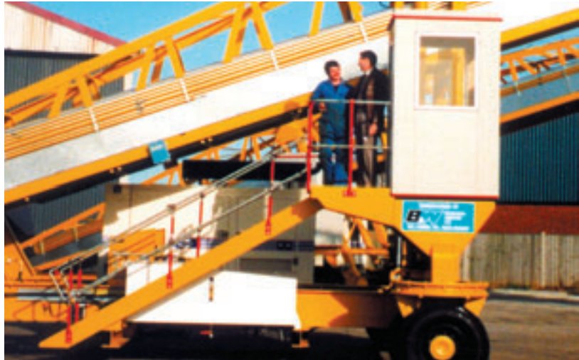
Operator's Control Cabin raised above the Forward Axle
