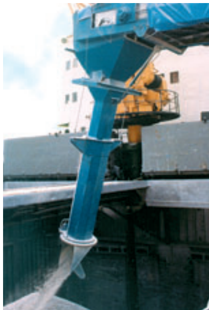
Two stage variable angle and telescopic trimming chutes
