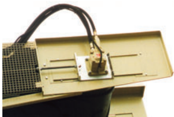
Integral Hydraulic Motor Drive to the Head Pulley
