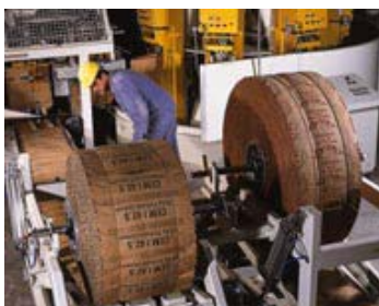
The double reel magazine allows the change of rollers with ongoing filling
