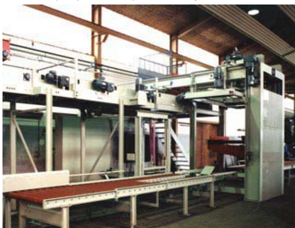
Palletizer with pile-up line for filled pallets, served by forklift
