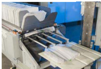
Fully automatic feeding of the empty bag bundles – high productivity is guaranteed
