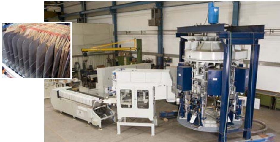
6-spout air-rotary packer with bag applicator and cassette magazine during testing in works.
