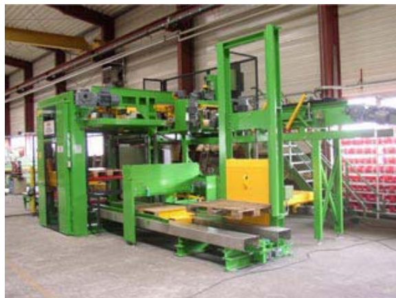
Palletizer with empty pallets magazine and bag conveyor
