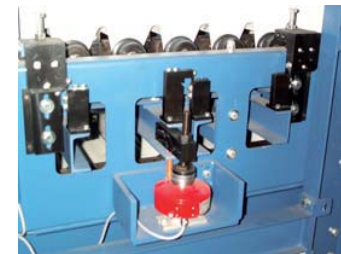
Weighbridge Digital load cell
